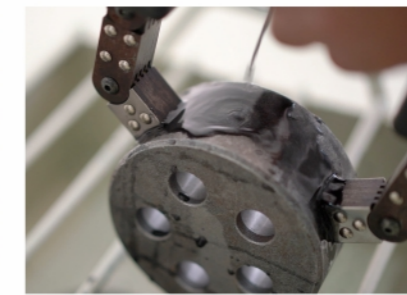
Anchorage Magnetic Particle Inspection
