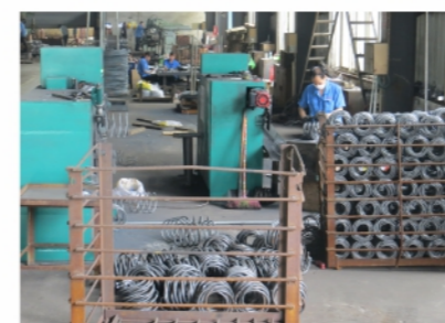
Spiral Reinforcement Production Line
