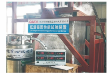
Low Temperature Anchoring Performance Test
