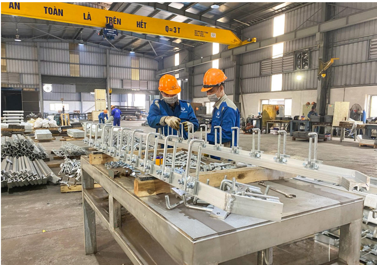
Production of the VHAL Aluminum-Alloy Rail Expansion Joint at Vinh Hung Factory
